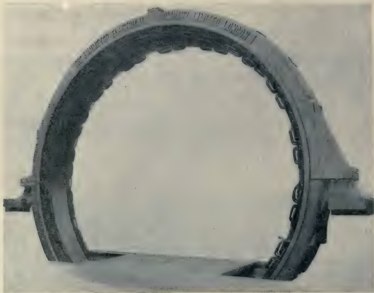
FIG. 255.—Armature of Lahmeyer 4000 k. w. 10,000-volt Alternator. Thirty-six-pole, Three-phase, Whole-coiled, Double-coil, Four-slot Spiral Winding in three ranges.
